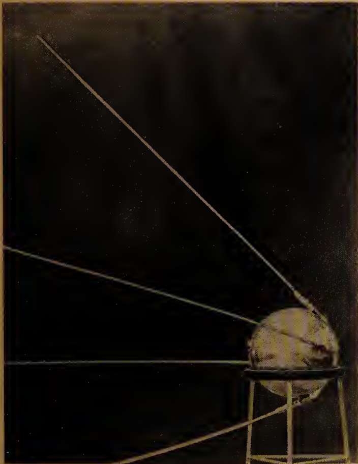
This official photo of the satellite Sputnik 1 was released by the Soviet government in Moscow. The satellite rests on a stand, and its four antennae can be seen projecting from the main structure of the satellite.
